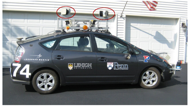
Fig. 3. Experimental test bed for LIDAR calibration experiments. Ben integrates an OXTS RT-3050 for 6DoF vehicle pose estimation, and a pair of roof mounted vertically scanning Sick LMS291-S14 LIDARs (circled red) to capture relative range measurements.
