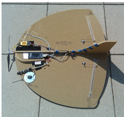
Fig. 1. Uglo 6 development platform used in this work. During testing, the aircraft was flown manually while telemetry data were logged via the on-board Piccolo SL autopilot system.
