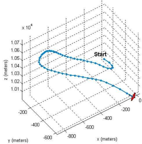
Figure 4: Dynamic soaring trajectories for optimizing solar exposure at midday. Note that minimizing the aircraft incidence angle to the sun results in a dramatically different trajectory to the sunrise mission due to significant changes in the solar altitude/azimuth.
