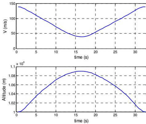
Figure 3: Aircraft velocity (top) and altitude (bottom) vs. time for the sunrise trajectory. The exchange of velocity for altitude is characteristic of the dynamic soaring cycle.
