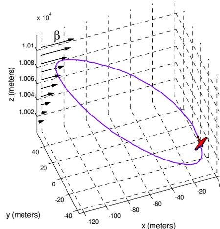
Figure 1: A dynamic soaring trajectory for loitering. The aircraft climbs into the wind gradient  $\beta$  to gain altitude, and dives with the wind to gain velocity. The energy obtained from such a trajectory can support perpetual flight.
