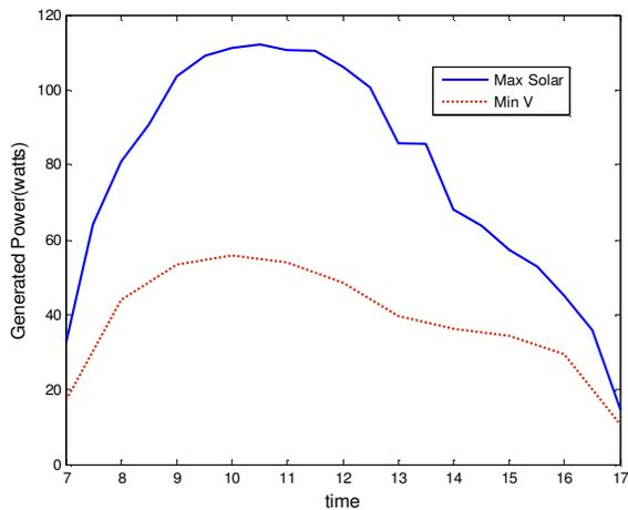
Figure 3: Power generated vs. time of day for trajectories optimizing velocity (bottom) vs. solar power (top). The average power generated over the 24 hour period was 16.1 and 32.6 watts, respectively.
