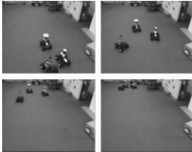
Figure 14: Trajectory for two pursuer robots tracking a moving target robot in an obstacle-free environment.
