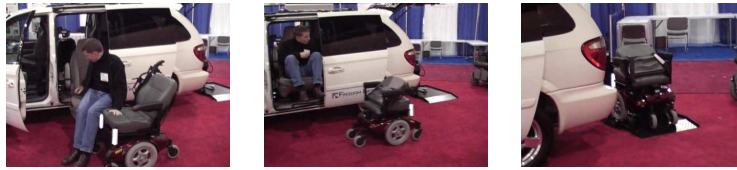
Fig. 5. ATRS demonstration at WCD2006. The operator performs a seat-to-seat transfer (left), and then remotely controls the wheelchair to the vicinity of the lift platform (center). At this point, the LIDAR tracks the chair while sending real-time control inputs over a dedicated RF link. Autonomous operations conclude with the chair successfully docked (right).
