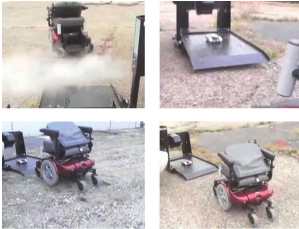
Figure 21. (Clockwise from upper left): Docking trials with vehicle exhaust for laser interference and the lift platform elevated, on broken asphalt, and on a sand and gravel surface. The wheelchair successfully docked in each of these trials.
