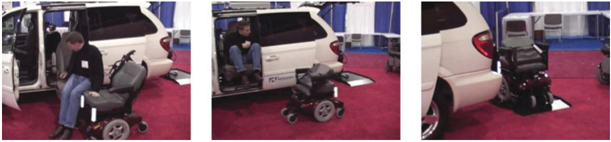
Figure 19. ATRS demonstration at WCD 2006. The operator performs a seat-to-seat transfer (left), and then remotely controls the wheelchair to the vicinity of the lift platform (center). At this point, the LIDAR tracks the chair while sending real-time control inputs over a dedicated RF link. Autonomous operations conclude with the chair successfully docked (right).
