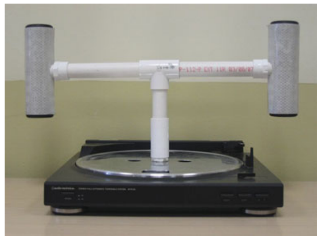
Figure 9. Test fixture used throughout localization subsystem testing. The turntable modeled wheelchair motion while allowing the simulated wheelchair position estimates to be projected to a single point.
