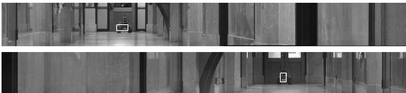
Fig. 6. Partial mosaic from the images acquired during a link acquisition trial. Using an 18X optical zoom, each robot was able to accurately localize its link partner at a range of \approx 45 meters to enable fast FSO link acquisition.
