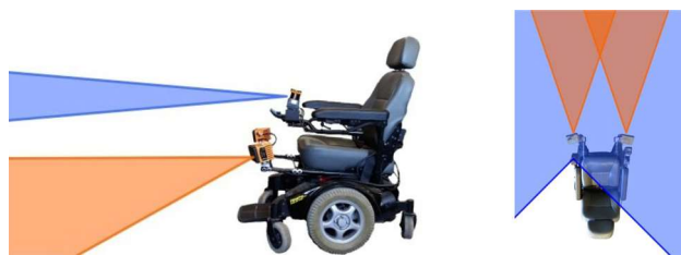
Fig. 9 The SWS prototype with the fields of view of the actuated LIDAR (blue) and each 3D camera (orange) highlighted. A profile view (left) and a top down view of the respective sensors' fields of view (right) (Color figure online)
