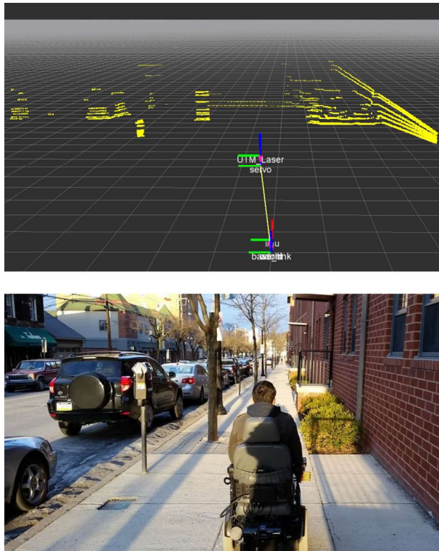
Fig. 11 A scan from the 3D Hokuyo ( top ). A photo of the corresponding scene ( bottom ). Clusters in the former from landmark poles are clearly visible
