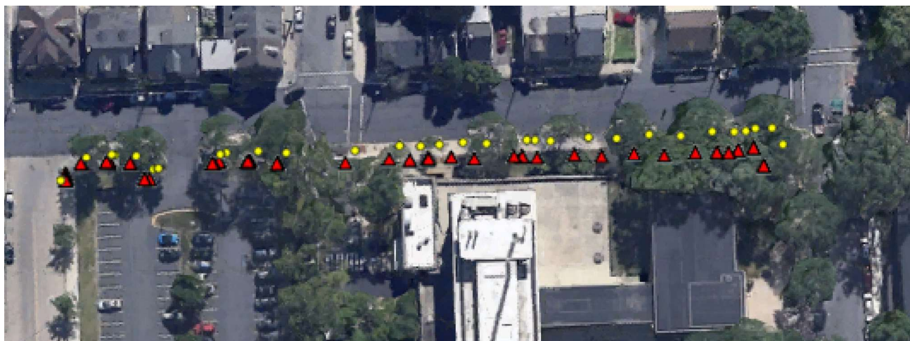
Fig. 8 A comparison of an initial landmark map to the refined map. The trike started on the left with an acceptable GPS position estimate and traveled to the right up a grade of 8.5%. The red triangles indicate the landmarks in M_{v1} and the yellow circles indicate the landmarks
