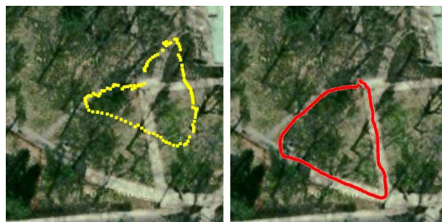
Fig. 2 A demonstration of the ineffectiveness of GPS as method of sidewalk level localization. The GPS signal is overlaid on satellite imagery while driving around the triangular-shaped path (left). The path derived from SLAM using trees as landmarks (right)
